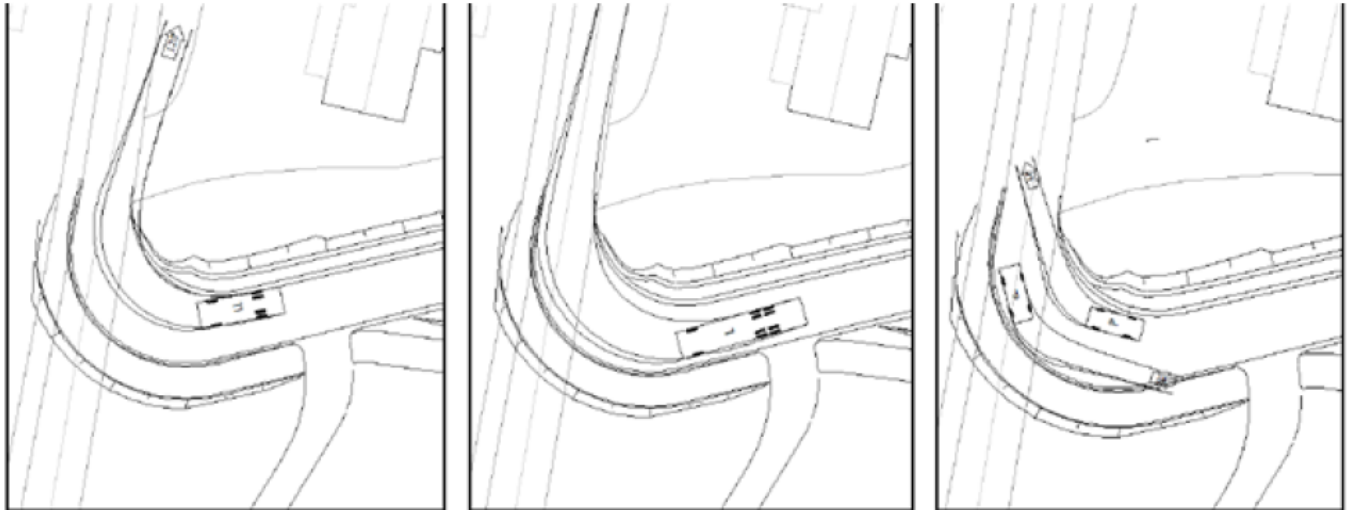
Figur 2: T.v. springkurve for Liten bil, midten springkurve for lastebil 12m, t.h. springkurve personbil
